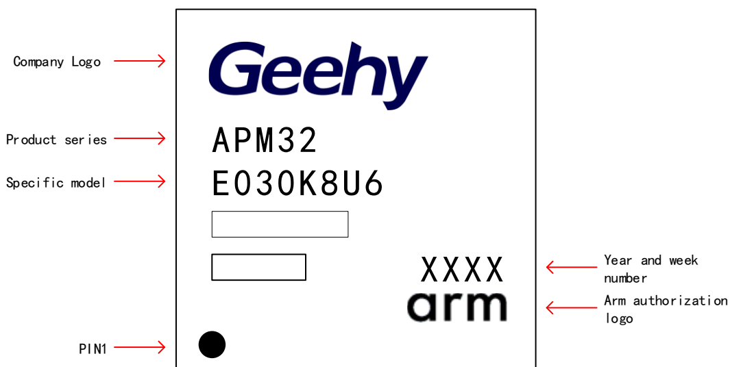
Figure 34 QFN32 - 32 Pins, 5 x 5mm Package Schematic Diagram
