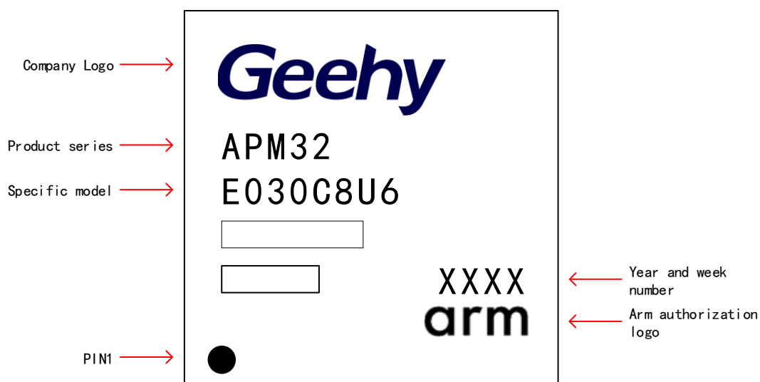
Figure 28 QEN48 - 48 Pins, 7 x 7mm Package Schematic Diagram
